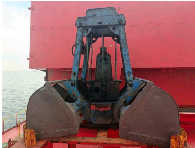
Gambar 1. Hydraulic Grab MV. Nashalina Sumber: Dokumentasi Peneliti (2024)
