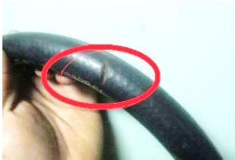
**Gambar 4.** Kebocoran High Press Hose
