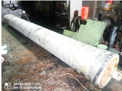
**Gambar 6.** Membran Fiber Mikron
