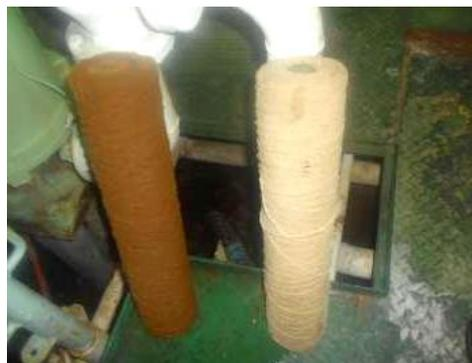
**Gambar 5.** Micron Fiber Kotor
