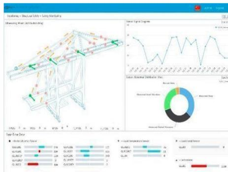
Gambar 4. *Real-time monitoring function interface of steel structure*
