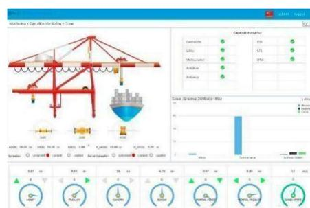
Gambar 6. *Real-time monitoring interface of single port crane*
